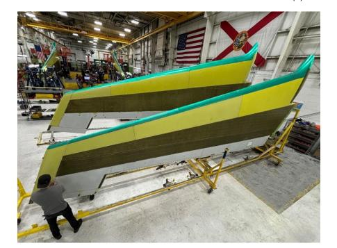
Daher Aerospace's assembly of aerostructures at Witham Field include horizontal stabilizers for Boeing 767 jetliners and the U.S. Air Force KC-46 aerial tanker version. (Photo: © Daher Aerospace)
